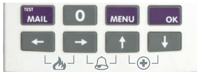
Figure 14: Keypad Emergency Alarm Trigger's
